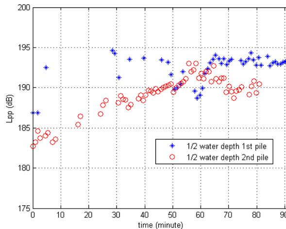
Figure 6: Peak-to-peak level (Lpp) for single strike of piling noise against piling time, recorded at 1/2 water depth. Piling operations lasted ca. 92 minutes for the 1st pile and ca. 80 minutes for the 2nd pile.
