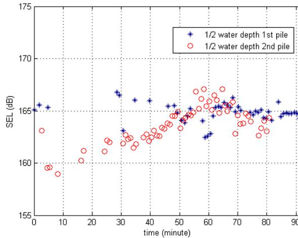
Figure 5: Sound Exposure Level (SEL) for single strike of piling noise against piling time, recorded at 1/2 water depth. Piling operations lasted ca. 92 minutes for the 1st pile and ca. 80 minutes for the 2nd pile.
